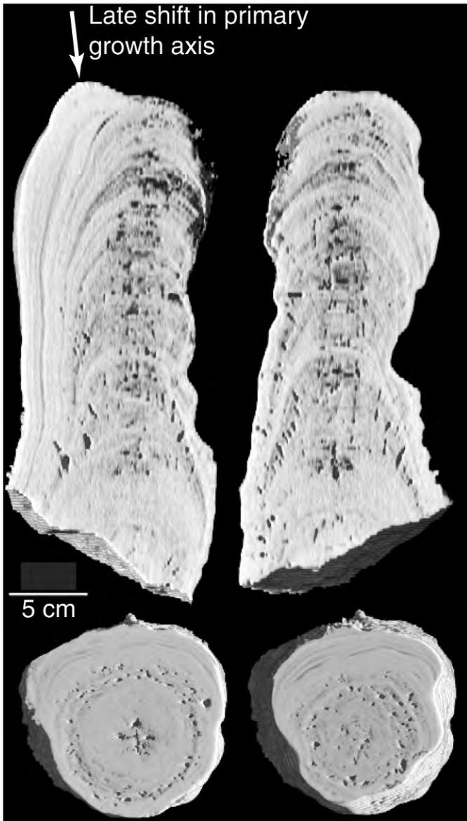
**Figure 3. Volume renderings of ANY-01. Cutaways reveal a late shift in the primary growth axis and significant internal porosity around the growth axis. Calcite deposited after the shift in the growth axis has a significantly lower porosity and higher density than calcite near the core of the speleothem. This calcite drape further complicates the visual inspection of the speleothem by obscuring the highly porous central core.**
