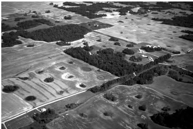
Figure 2. Aerial view of a typical area within the southwestern Illinois sinkhole plain adjacent to the bluffs of the Mississippi River looking west. Sinkholes are marked by depressions, tree clusters, and ponds. Photograph by Joel Dexter, ISGS, 2000.
